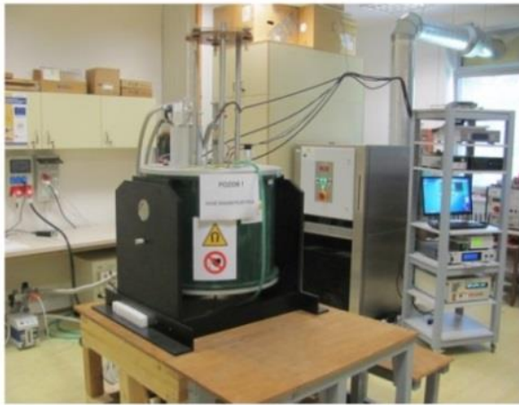
Experimental facilities for thermal processing of materials in high magnetic fields (up to 14 T)
