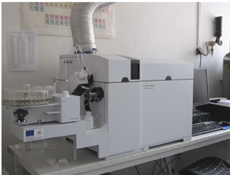
ICP-MS spectrometer Agilent 7700 for element detection in the range of 2–260 amu, a possibility ultratrace analysis with sensibility of ppt units
