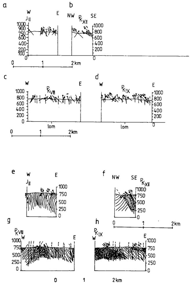
Fig. 4. Profiles along the vertical electric sounding cross sections J<sub>II</sub>, P<sub>KVII</sub>, P<sub>KIX</sub>, P<sub>KXII</sub>, made by Spěváková & Valušáková (1986) through the Bystrica and Beloveža Formations, indicated in Fig. 1b. a, b, c, d - raw data; e, f, g, h - interpretation, blank - sediments of the Bystrica Formation, dot pattern - sediments of the Beloveža Formation. See Fig. 2 for an explanation.
