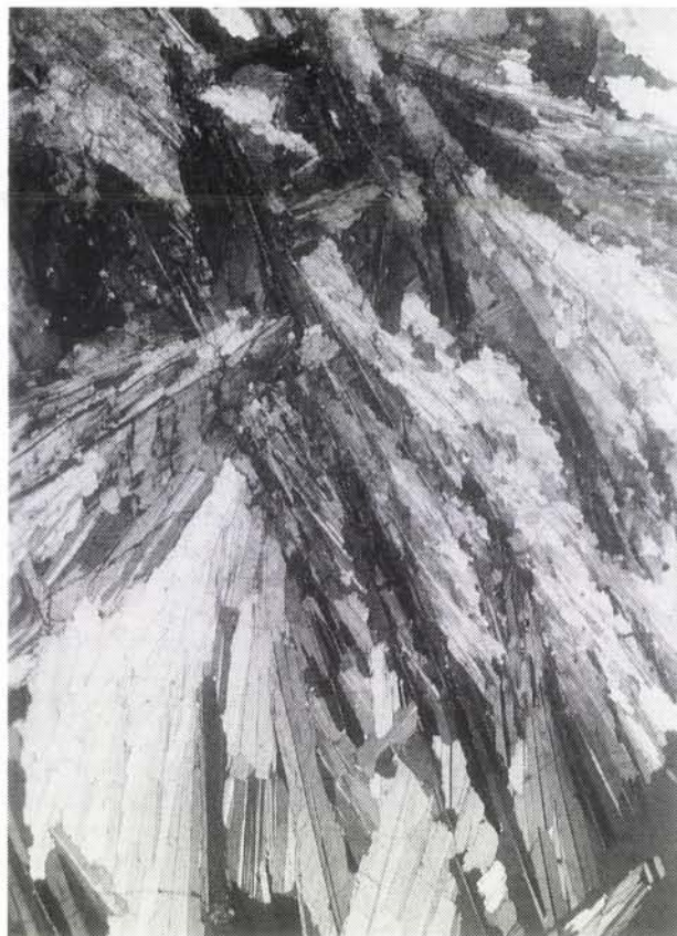
Fig. 13. Tabular crystals of cleavelandite with a fan-like arrangement, from the albite zone. Striebornica sample 33h. Microphoto magnification 8.5x, crossed nicols.
