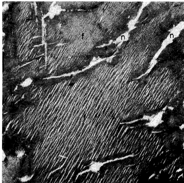
Fig. 2. Film to short spindle perthites of exsolutional origin (f) with irregularly patchy perthites (n). Block zone pegmatites. Quarry in Hradná Valley sample 23b. Microphoto magnification 130x, crossed nicols.
