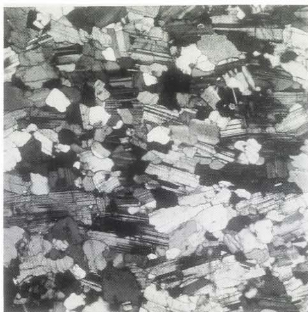
Fig. 12. Granular, saccharoidal albite with albite and albite - Karlsbad twinning from the albite zone. Striebornica sample 33h. Microphoto magnification 35x, crossed nicols.
