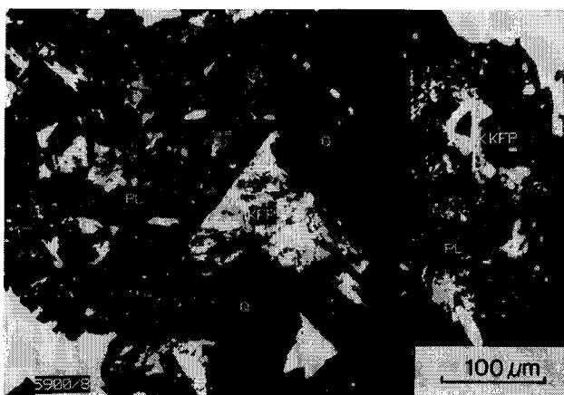
Fig. 2b. Back-scattered electron image of zoned plagioclase in quartz groundmass (An 72 - An 55 - An 22 ).
