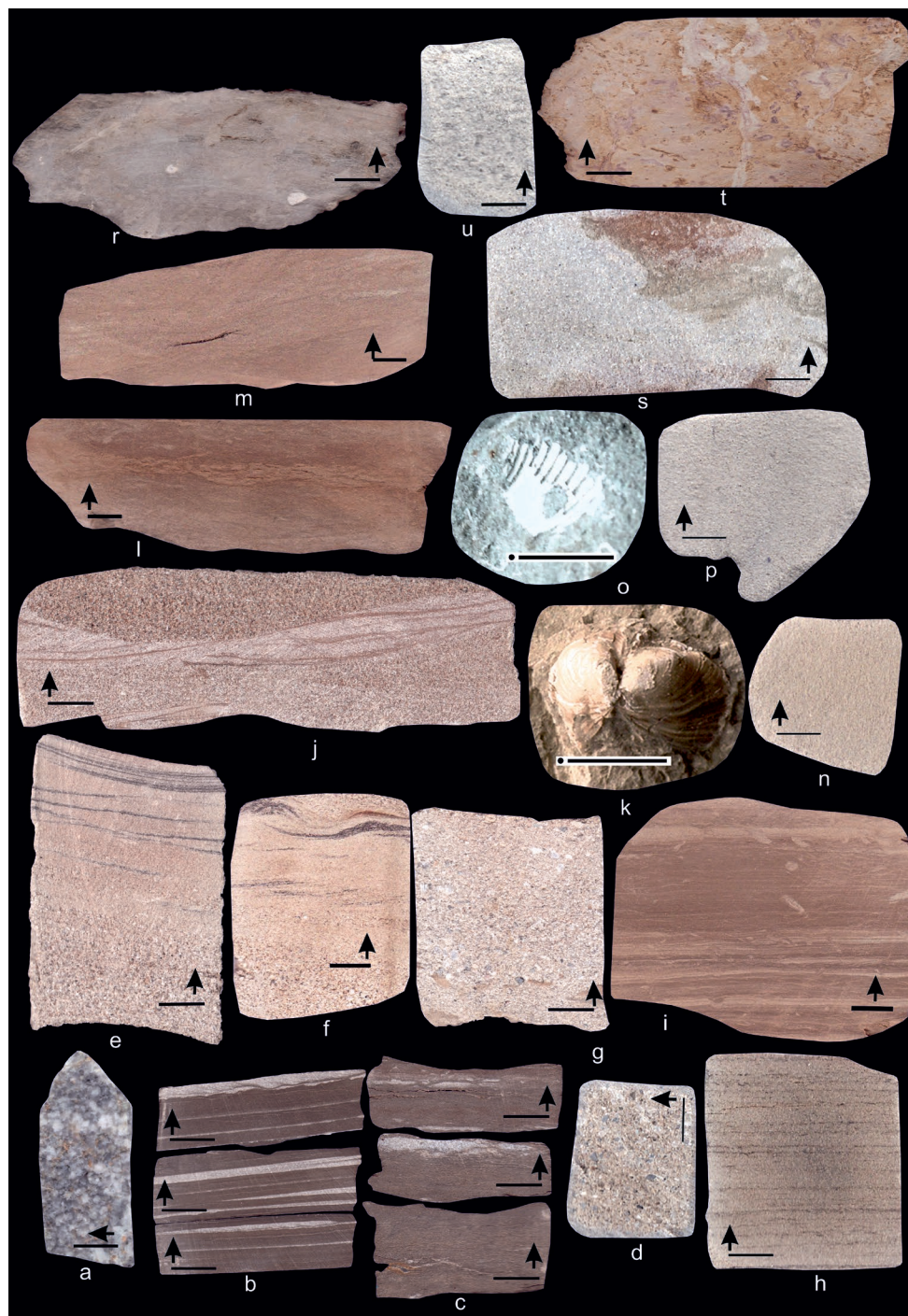
Fig. 5. MOJ-1 well core samples (scale bar = 1 cm, arrow pointing upwards, dot = bedding plane): a — leucocratic granite; MOJ-1/c33, 2095–2100 m/b2; b — heterolithic sediment with lenticular sandy ripples; MOJ-1/c31, 2005–2010 m/b2; c — heterolithic sediment with sandy ripples; MOJ-1/c27, 1795–1798,5 m/b5; d — poorly sorted conglomerate with poorly rounded clasts reach 2–3 mm in diameter; MOJ-1/c27, 1795–1798,5 m/b5; e — fluent transition from normally graded sandstone through laminated sandstone to sandy ripples which are draped by carbonized plant fragments (gravity flow sediment); MOJ-1/c25, 1705–1710 m; f — the same as e, but with an erosive contact on the top; MOJ-1/c25, 1705–1710 m/b1; g — normally graded coarse-grained sandstone to conglomerate (max. 2–5 mm diameter) with mudstone intraclasts; MOJ-1/c25, 1705–1710 m/b4; h — laminated, fine-grained sandstone. Laminae are formed by carbonized plant fragments; MOJ-1/c22, 1551–1556 m/b1; i — bioturbated mudstone with sporadic sandy laminae; MOJ-1/c18, 1351–1354 m; j — medium-grained sandstone ripples forming flaser bedding; MOJ-1/c17, 1298–1303 m/b4; k — Congerina cf. czjzeki Hörnes. MOJ-1/c16, 1253–1261 m/b6; l — indistinctly bioturbated mudstone; MOJ-1/c16, 1253–1261 m/b5; m — massive mudstone with carbonized plant fragments; MOJ-1/c13, 1099–1104 m/b1; n — massive sandstone; MOJ-1/c12, 1054–1059 m/b2; o — Cardiidae indet.; MOJ-1/c11, 1000–1005 m/b4; p — massive, medium-grained sandstone; MOJ-1/c11, 1000–1005 m/b2; r — mudstone with sandy concretions, red mottles and rhizoids; MOJ-1/c10, 955–960 m/b4; s — massive, medium-grained sandstone with a reddish mudstone intraclast; MOJ-1/c5, 703–708 m/b1; t — mudstone with red mottles, and rhizoids; MOJ-1/c4, 649–654 m/b2; u — massive medium-grained sandstone; MOJ-1/c2, 549–554 m/b2.
