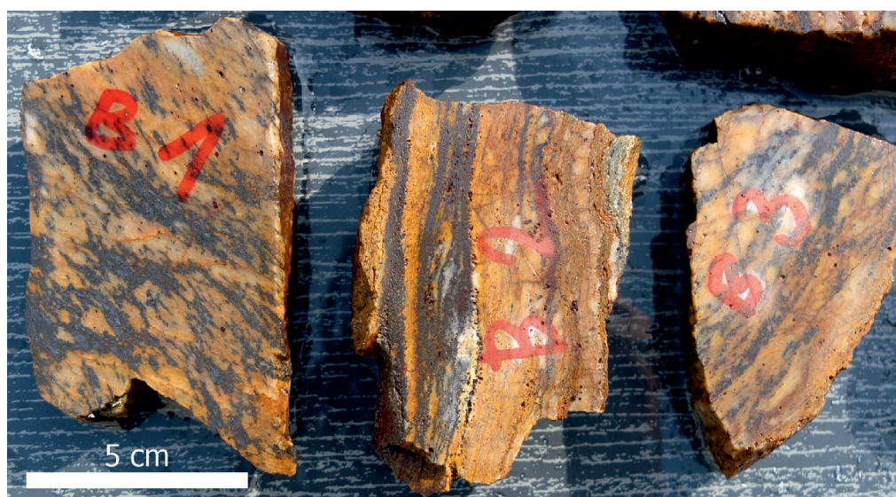
Fig. 6. Hand specimens from Bacúch, showing the magnetite bands in quartz.
