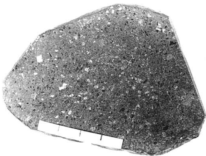
Fig. 9. Radiogram of quartz porphyry pebbles (dark) in tuffite conglomerate, Novoveská Huta, scale 2 : 1. Photo T. Mastihuba
