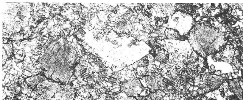
Fig. 16. Corrosion of dolomite rhombohedrons by calcite. The big quarry Polom, Small Fatra. Magn. 55X. Photo by L. Osváld.
