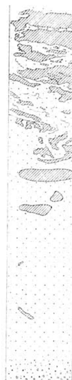
Fig. 10. Graded sandstone with slump structures on the top. Gradual transition from graded turbidite into slump is noteworthy. Borehole B-85, 150.90 m.
