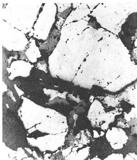
Fig. 23. Fractured pyrite surrounded and veined by chalcopyrite (light grey), sphalerite (medium grey), Quartz and chlorite (dark grey). Copper rich pyrite ore, Smolnik. Polished section, 100 X.
