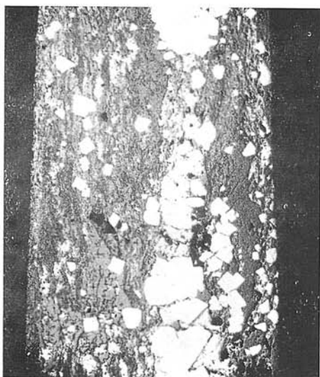
Fig. 17. Chalcopyrite-pyrite band (coarse grained) in disseminated ore. Smolnik. Sample 173. Polished section, 4 X.
