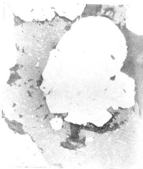
Fig. 24. Pyrite sphere overgrown by idio-blastic pyrite. Sphalerite containing numerous chalcopyrite blebs. Compact chalcopyrite-pyrite ore. Smolník. Polished section, 320 X.
