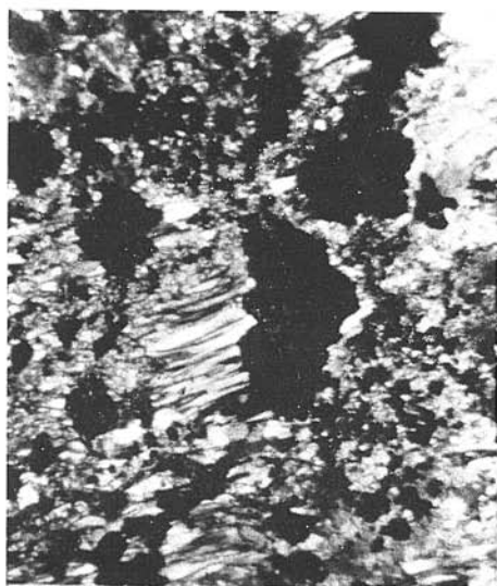
Fig. 22. Pyrite aggregates with quartz in pressure shadows. Smolnik. Thin section, Nicols X, 32 X.
