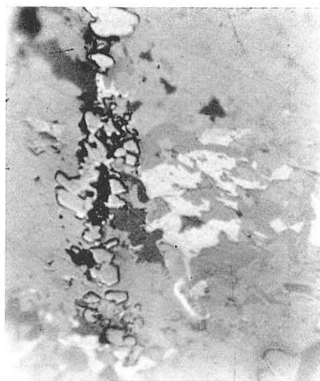
Fig. 29. Native bismuth (white) with bis-muthinite in chalcopyrite. Arsenopyrite lining a fracture. Compact Cu-ore. Smolník. Polished section, 1000 X.
