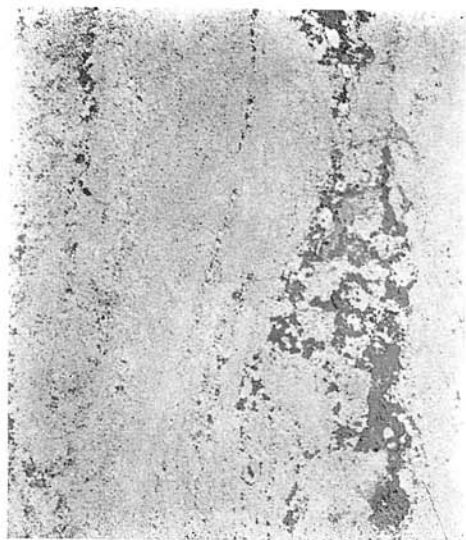
Fig. 6. Compact pyrite ore with coarser recrystallized pyrite lining quartz-carbonate lenses containing chalcopyrite, sphalerite etc. Smolník. Polished section, 4 X.
