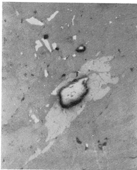
Fig. 5. Amphibolite impregnated by pyrrhotite (white). Ilmenite (light grey, relief), surrounded by rutile (light grey). Polished section, 150X.
