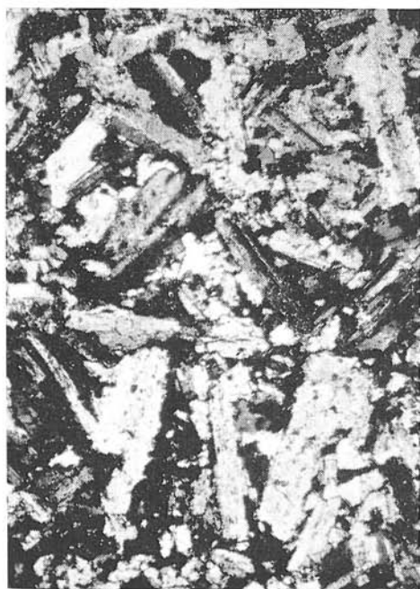
Fig. 3. Porphyrite with the laths of plagioclase and chlorite (Košická Belá, crossed nicols, 45 X, photo H. B r o d ě n s k á).
