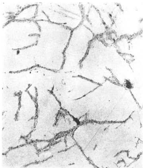
Fig. 5. Hexagonal pyrrhotite in initial stage of replacement by monoclinic modification (dark-grey) along fissures and grain boundaries. Covered with magnetite suspension. Pezinok, borehole PZ-62, polished section, magnif. 150 X
