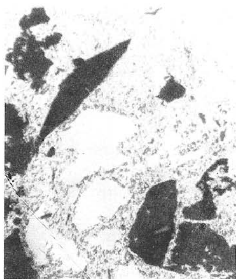
Fig. 6. Relics of hexagonal pyrrhotite (light-grey) in monoclinic pyrrhotite (light-darker-grey spotted, covered by magnetite powder) Amphiboles, quartz — blackish-grey. Pezinok, borehole PZ-62, polished section, magn. 150 X.
