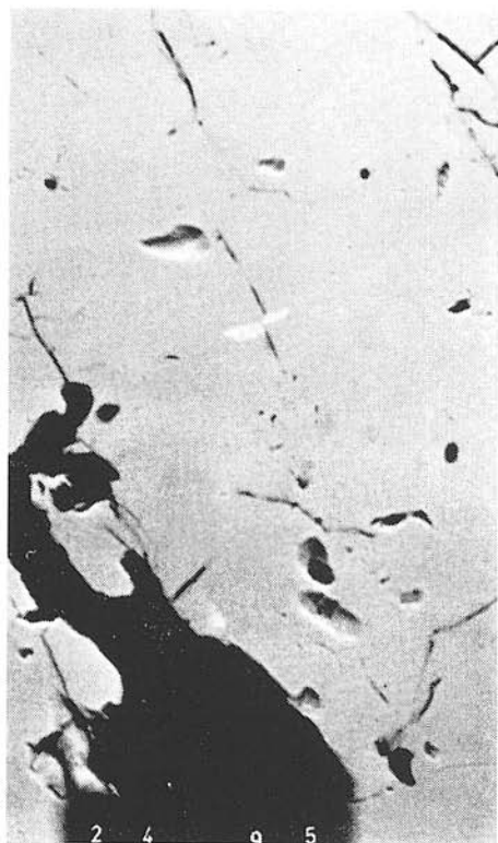
Fig. 11. Hexagonal pyrrhotite with common type bush-shaped pentlandite. Bratislava, quarry in the Vydrica Valley, polished section, magnif. 1300 X.
