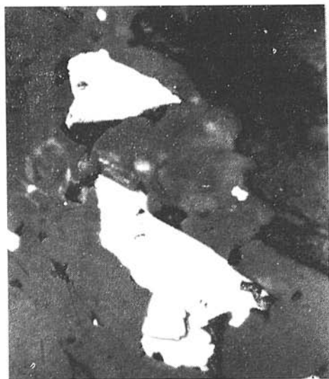
Fig. 13. Pyrrhotite-pyrite impregnations in amphibolite. In pyrrhotite elongated pentlandite. Locality like in fig. 11. Polished section, magn. 600 X.
