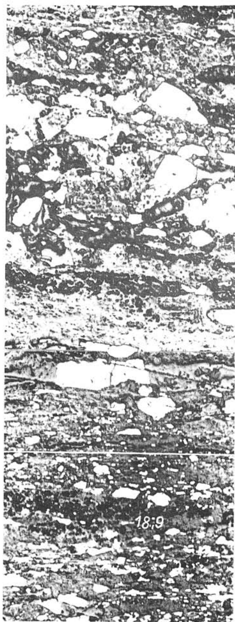
Fig. 12. Idiomorphic pyrite in wedged-shaped pyrite-schistose bands. Detail from lower part of Fig. 10. Polished section, magn. 12 \times .
