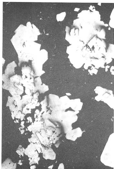
Fig. 25. Arsenopyrite (relief) enclosed in gudmundite. Carbonates — black. Polished section, magn. 150 X.
