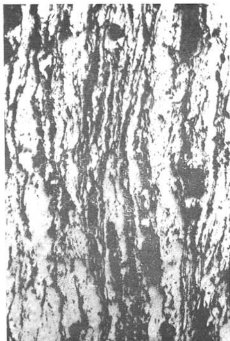
Fig. 13. Common type of thinly-laminated pyrite from pyrite-quartz band. No plastic deformation. Polished section, magn. 150 X.
