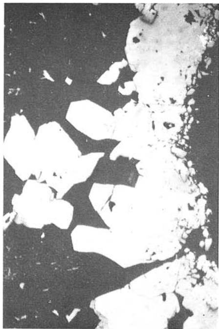
Fig. 24. Coarser gudmundite rimming earlier, fine-grained arsenopyrite (relief). Polished section, magn. 150 X.
