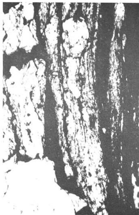
Fig. 14. Contact of laminated (gray) and crystalline (white) pyrite. Etched with \text{KMnO}_4 + \text{H}_2\text{SO}_4 . Colloform deposited pyrite in the laminae is readily attacked by etching. Polished section, magn. 150 X.
