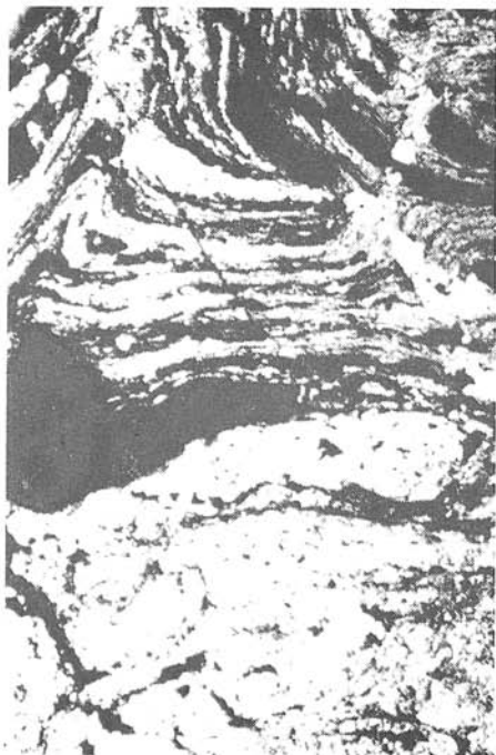
Fig. 15. Microfolds in laminated pyrite. Initial stage of crystallization. Etched with \text{KMnO}_4 + \text{H}_2\text{SO}_4 . Polished section, magn. 150 X.
