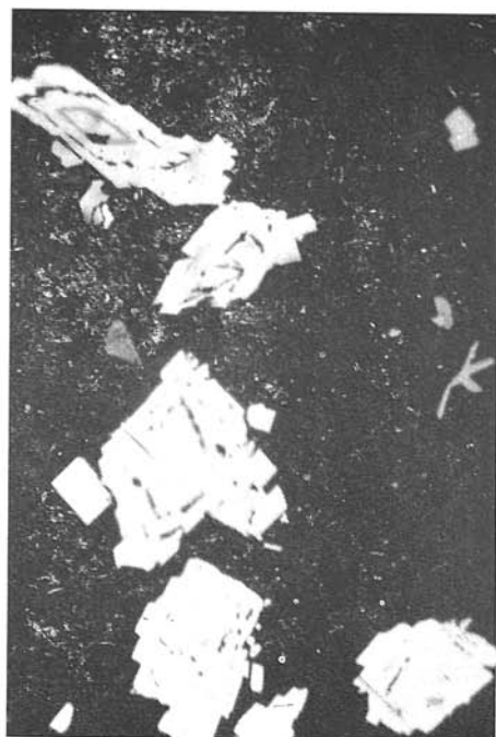
Fig. 22. Zonal arsenopyrite in carbonate. Polished section, magn. 450 X.
