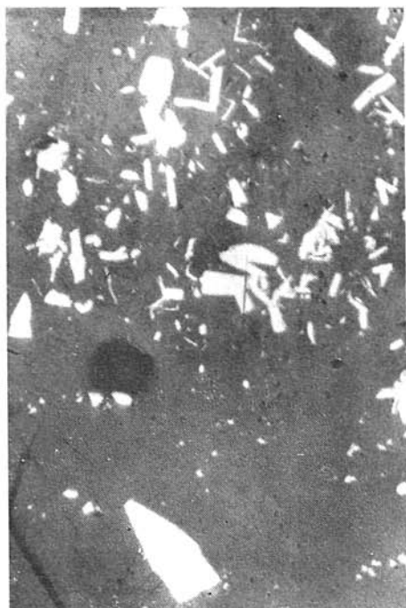
Fig. 26. Idiomorphic crystals of monoclinic pyrrhotite in carbonate. Larger gudmundite near lower edge of the photograph. Polished section, magn. 220 \times .
