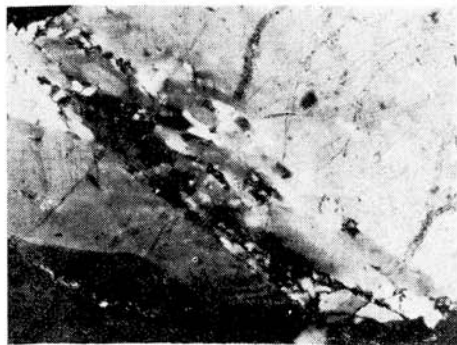
Fig. 9. Monocrystalline undulatory grain with new small quartz crystals along the zones of discontinuity. Loc. Donovaly, Nízke Tatry Mts., s. 7, X nicols, magn. 43 X. Photo C. Michalíková.
