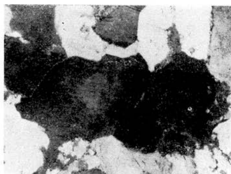
Fig. 11. Monocrystalline undulatory quartz with undulatory oriented overgrowths. Loc. Smrekovec, Malá Fatra Mts., s. 5, X nicols, magn. 43 X. Photo C. Michalíková.
