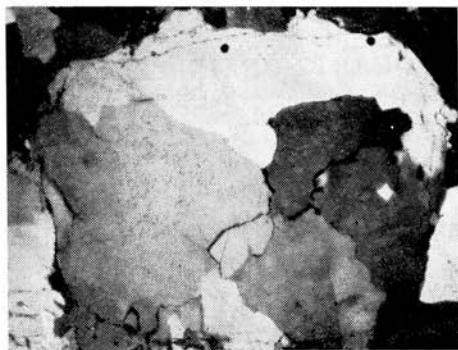
Fig. 2. Polycrystalline grain from massive plutonic rocks with undulatory oriented overgrowth. Loc. Lipt. Lúžna, Nízke Tatry Mts., s. 150, X nicols, magn. 43 X. Photo C. Michalíková.
