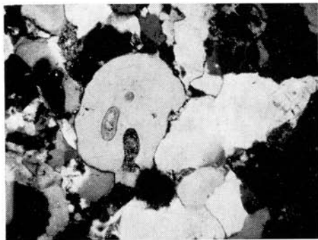
Fig. 5. Monocrystalline quartz from effusive rocks, it has bipyramidal habitus and preserved features of corrosion and inclusions. Loc. Lipt. Lúžna, Nízke Tatry Mts., s. 174, X nicols, magn. 43 X. Photo C. Michalíková.
