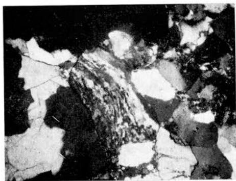
Fig. 3. Fine-polycrystalline grain from gneisses. Loc. Lipt. Lúžna, Nízke Tatry Mts., s. 4, X nicols, magn. 43 X. Photo C. Michalíková.
