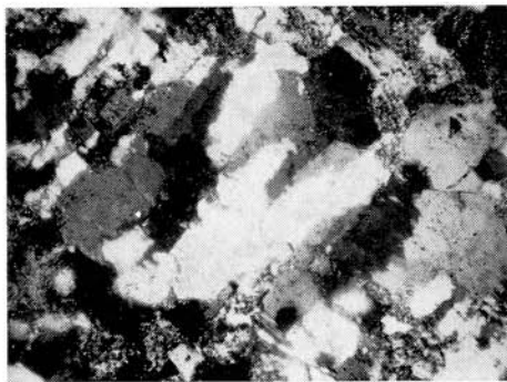
Fig. 7. Vein quartz from small vein in quartzite. Loc. Lipt. Lúžna, Nízke Tatry Mts., s. 190, X nicols, magn. 43 X. Photo F. Martančík.
