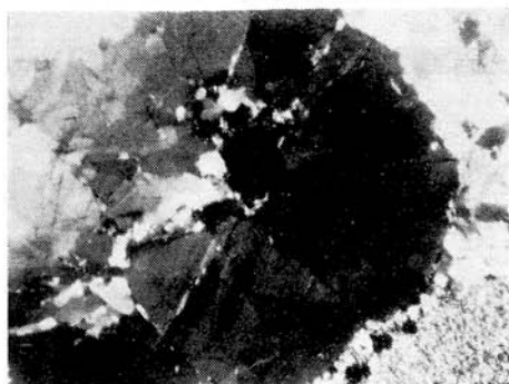
Fig. 10. Monocrystalline undulatory quartz, the zones of discontinuity can be very well seen. Loc. road-cut to Srdiečko, Nízke Tatry Mts., X nicols, magn. 43 X. Photo C. Michalíková.
