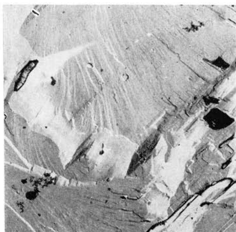
Fig. 15. Grained antimonite, Kremnica, sample 3, magnif. 7000 X. Aggregates of cinnabarite of minute dimensions and individual crystals. Inclusions of other minerals (grey) are also to be seen.
