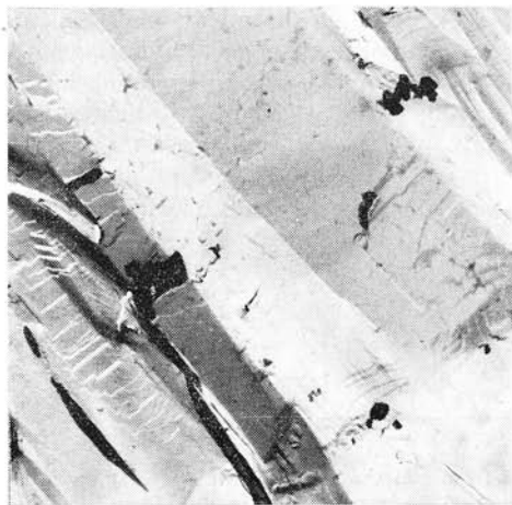
Fig. 6. Grained antimonite, sample 3, magnif. 7000 \times . Inclusions of cinnabarite (metacinnabarite) (black) of dimensions up to 1 \mu m. Explanations: Two-stage replica (Pt 80 %, Pd 20 %). The black places (impermeable for electrons) represent partly submicroinclusions of cinnabarite, partly parts of the fundamental mineral, which arose by their tearing off when making the preparation.
