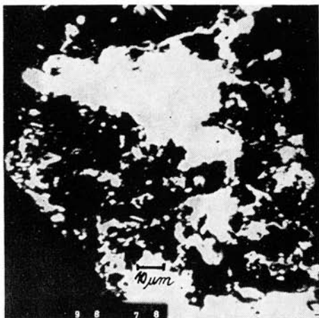
Fig. 20. Dve Vody, sample 26, magnif. 600 X. Composition of berthierite (somewhat darker) with antimonite (lighter-coloured).
