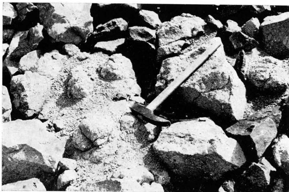
Fig. 11. Disintegration character of the propylitized pyroxenic andesite under conditions of extreme moisture and temperature changes in the rip-rap of the East Slovakian water reservoir dam in Fig. 10.
