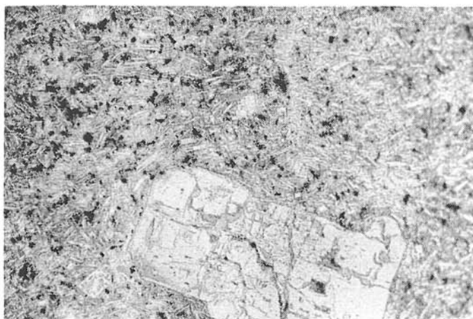
Fig. 6. Detail of groundmass texture from section 66 m from the upper stream. The microlites in the hyalopilitic groundmass flow around phenocrysts of plagioclases. The plagioclases contain many inclusions of mesostasis. Nicols //, magnif. 43 X. Photo by Martančík
