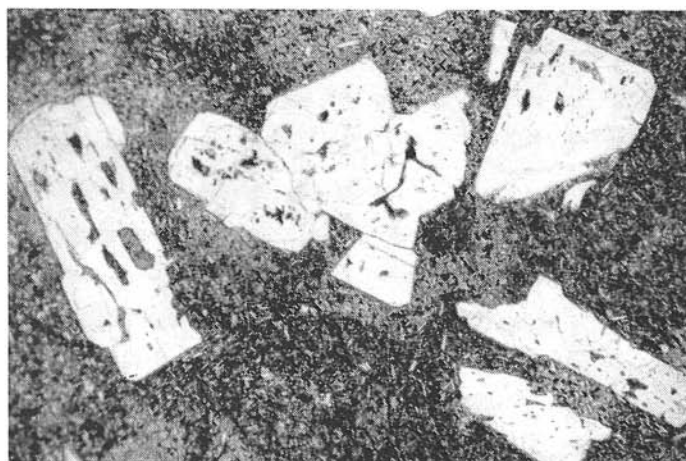
Fig. 5. Texture of groundmass from leucocratic andesite from 31,8 m is distinctly inhomogeneous. The inhomogeneity is caused by differentiation of the hyalopilitic groundmass into two parts; the lighter-coloured vitreous and darker, in which the vitreous mass is recrystallized into fibers and forms some imperfect spherulites among microlites of plagioclases. The plagioclase microlites are passing from one substance to other. Nicols //, magnif. 23 X. Photo by Martančík.
