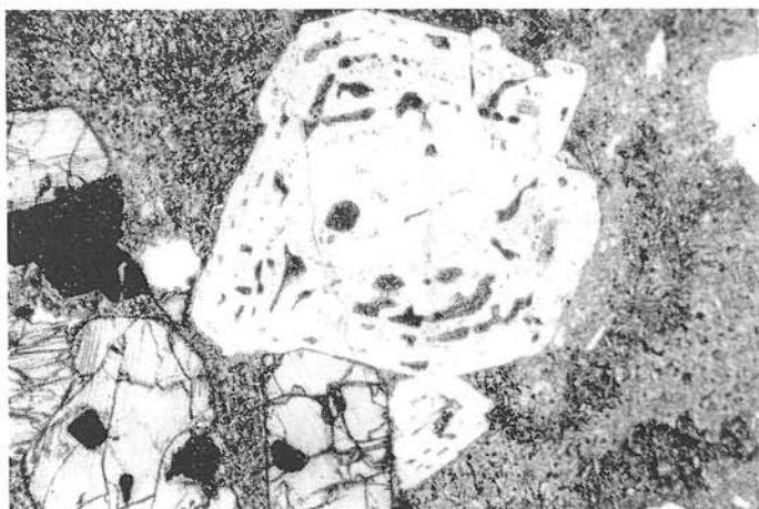
Fig. 4. 31,8 m. Porphyritic texture of leucocratic andesite from the upper stream in section 31,8 m. Characteristic in having large phenocrysts of plagioclases with many inclusions of mesostasis, from the cluster of pyroxenes and oxides (in the corner is twinned augite). The groundmass is hyalopilitic, inhomogeneous, Nicols //, magnif. 23 X. Photo by Martančík.
