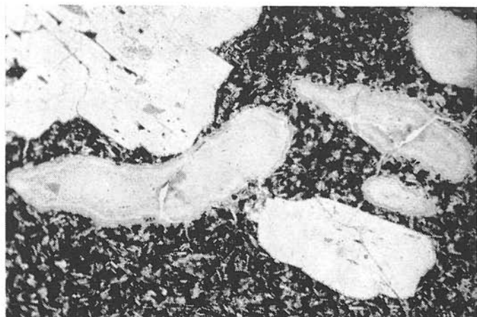
Fig. 12. Detail of groundmass from the basal part of the lower stream (section 149,5 m); among fluidally ordered phenocrysts are pores of elongated shapes with partial zonal filling. The microlites in the brown, vitreous groundmass are minute, thin, imperfectly developed. Nicols //, magnif. 43 X. Photo by Martančík.
