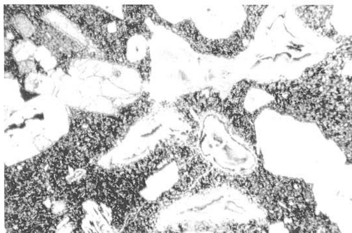
Fig. 11. Basal part of the lower lava stream (section 149.5 m), highly vesicular. The pores are of elongated shapes. They are filled up with various colloids of greenish, rusty-brown-greenish colours. The rock has weak fluidal arrangement. Nicols \parallel , magnif. 23 X. Photo by Martančík.
