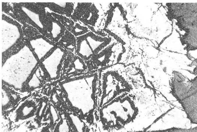
Fig. 11. Cataclastized chromium spinel (dark-grey), rimmed and filled in with magnetite (white) on cracks and with silicate minerals (light and medium grey). Jaklovce, reflected light, 80x, 1 nicol. Photo by I. Rojkovič.
