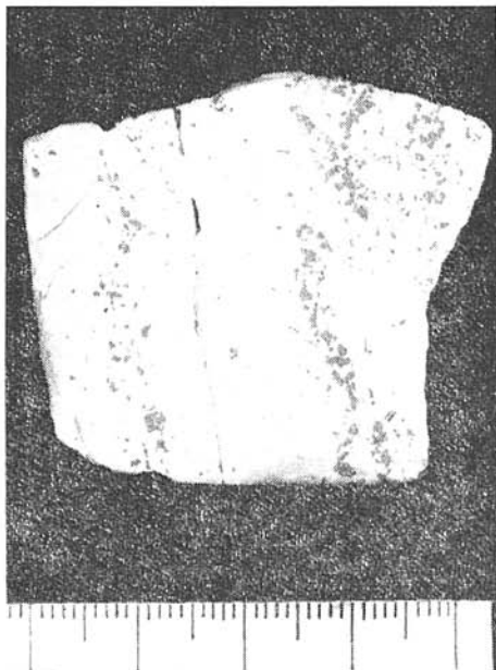
Fig. 5. Streaky parallel layers in serpentinite, enriched in chromite, Hodkovce, measure in cm. Photo by F. Martančík.
