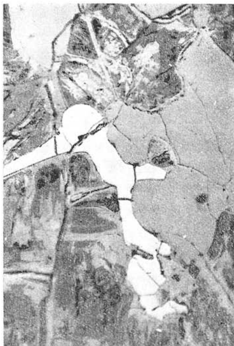
Fig. 20. Spinel (white) filling in the interstices of silicate grains in periodite xenolith. Mašková, reflected light, 160x, 1 nicol. Photo by I. Rojkovič.
