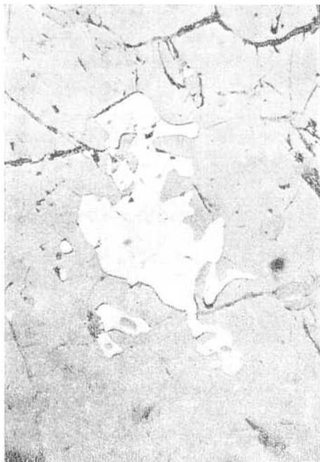
Fig. 2. Allotriomorphic spinel-ceylonite in amphibolic peridotite, Velká Lúka, reflected light, 160 x, 1 nicol. Photo I. Rojko-vič.
