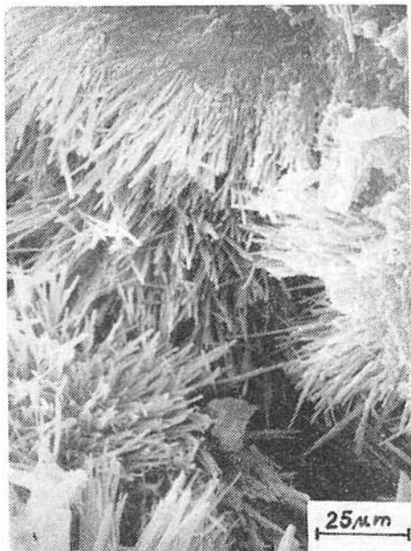
Fig. 13. Scanning electron microphotograph of monomineral aggregates of radiated mordenite from Bartošova Lehôtka.
