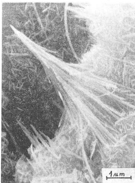
Fig. 14. Scanning electron microphotograph of fibers of mordenite with minute tables of cristobalite behind from Bartošova Lehôtka.
