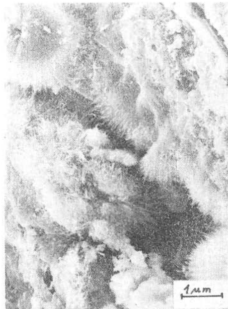
Fig. 15. Scanning electron microphotograph of fine-fibrous mordenite along a joint and on the edges of fragments of volcanic glass from Bartošova Lehôtka.
