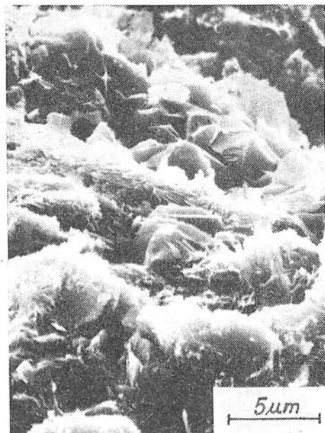
Fig. 2. Scanning electron microphotograph of fine-grained clinoptilolite zeolite from the quarry near Nižný Hrabovec.
