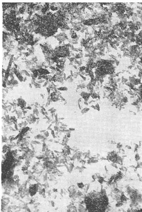
Fig. 2. Electron micrograph of halloysite, Slatinská kotlina basin, borehole SK-18/82,5 m, magnif. 18 000X.
