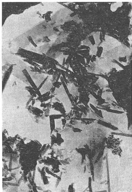
Fig. 3. Electron micrograph of halloysite and montmorillonite, Slatinská kotlina basin, borehole SK-25/27,2 m, magnif. 18 000X.
