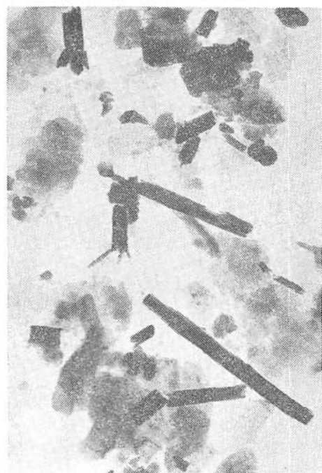
Fig. 6. Electron micrograph of halloysite ( 4\text{H}_2\text{O} ), Lučenecká kotlina basin, Kalinovo-Hrabovo, magnif. 50 000 \times .
