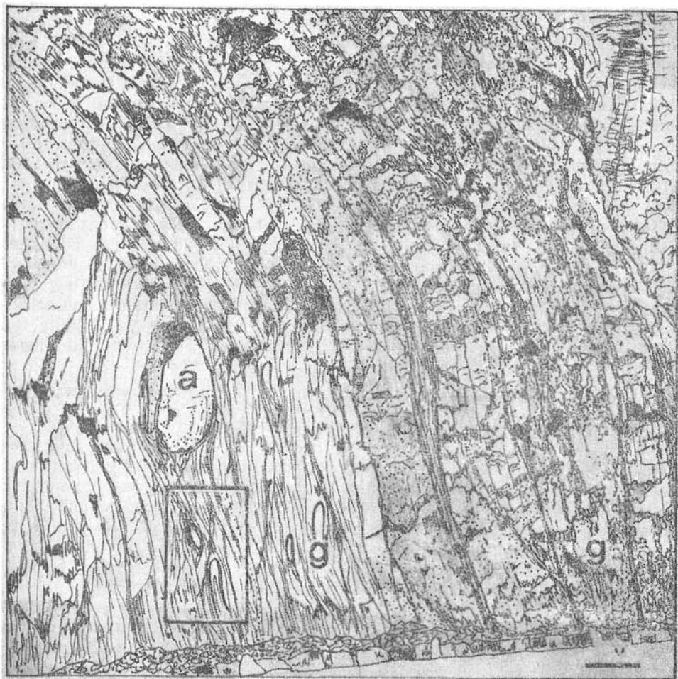
Fig. 4. Limb of isoclinal macrofold F_{2-1} with minor F_{1-1} in the left part (detail in frame see Fig. 3) and conform overprinting of s_{1-1} by s_{2-2} in the right part. Banded gneisses (g) and amphibolite gneisses (a) in the Bystrá valley.
