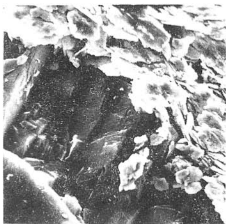
Fig. 3. Selective weathering of plagioclase lamellae. Biotite-muscovite granodiorite, Železná studnička — Bratislava. Scanning el. microscope, magnif. 4000 x.
