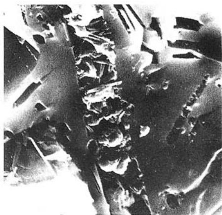
Fig. 2. Selective weathering of plagioclase lamellae. Biotite granodiorite of Prašivá type, (Sopotnica — Hronov). Scanning el. microscope, magnif. 14 000 x.
