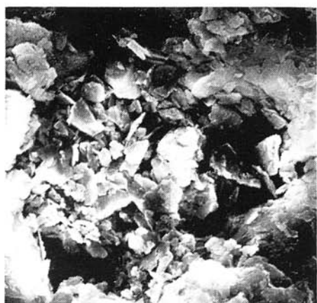
Fig. 6. Detail of "nest" of secondary minerals. Leucocratic hydro- (auto) metamorphosed granite, gamekeeper's cottage Horvátka, Borinka. Scanning el. microscope, magnif. 10 000 x.
