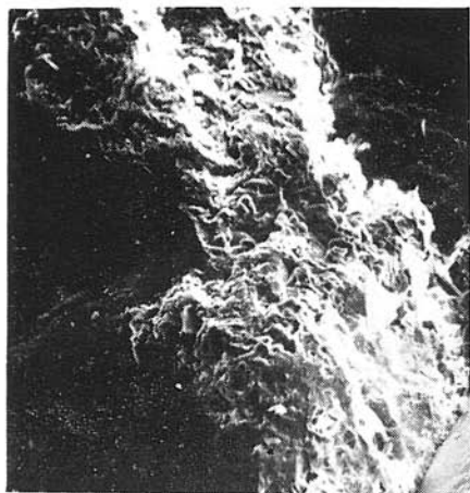
Fig. 1. Weathering of plagioclase — origin of secondary minerals transversely to lamellation. Tonalite — plagiogranite, Harmónia, quarry in the Zliabok brook. Scanning el. microscope, 4000 x.
