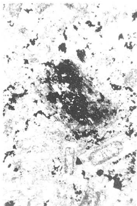
Fig. 3. Alabandite with pyrite (black) push back in the middle actinolitized and sericitized phenocrysts of pyroxenes in quartz diorite with abundant plagioclases. Víglášká Huta — Kalinka. Transmitted light, magn. \times 25 , 1 nicol.
