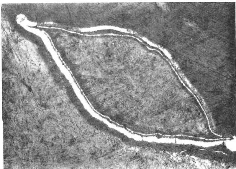
Fig. 2. Sealed Pt ampule lined by tungsten (thin open layer) in section. Glass (quenched andesite melt) is observed on the inside after a run at 1450 °C and 40 kbar.
