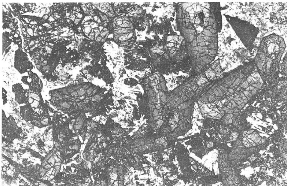
Fig. 9. Magnified 16.5 x with polarizer. Locality: Staříč — Kublův lom; teschenite clinopyroxenite with porphyritic texture. Zonal titan-augite phenocrysts enclose diopside relics.
