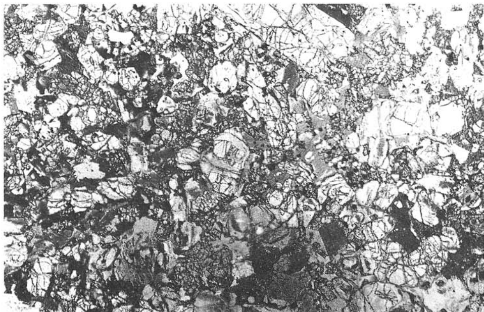
Fig. 6. Magnified 16.5 x with polarizer. Locality: Staříč — Kublův lom; granular picrite with poikilitic texture.
