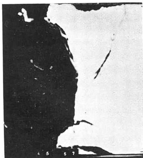
Fig. 14. Sample RB-51; a) composition of arsenopyrite II (light-coloured) and pyrite III (dark) (magn. 300X); b) areal As distribution in arsenopyrite II and pyrite III.
