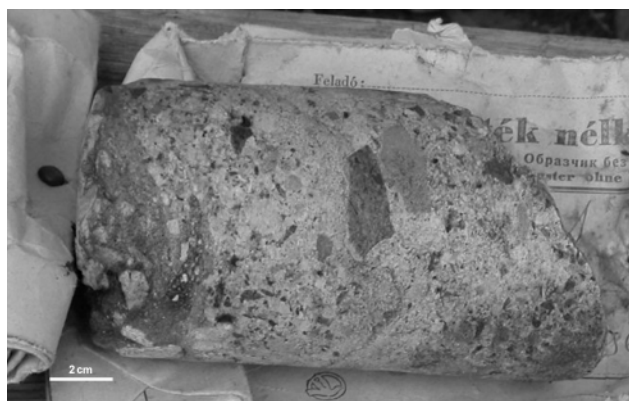
Fig. 4. Graded breccia sample from the Csehbánya-1 well, 396–398 m interval, with a chert fragment of 2 cm in diameter in the middle of the core.
