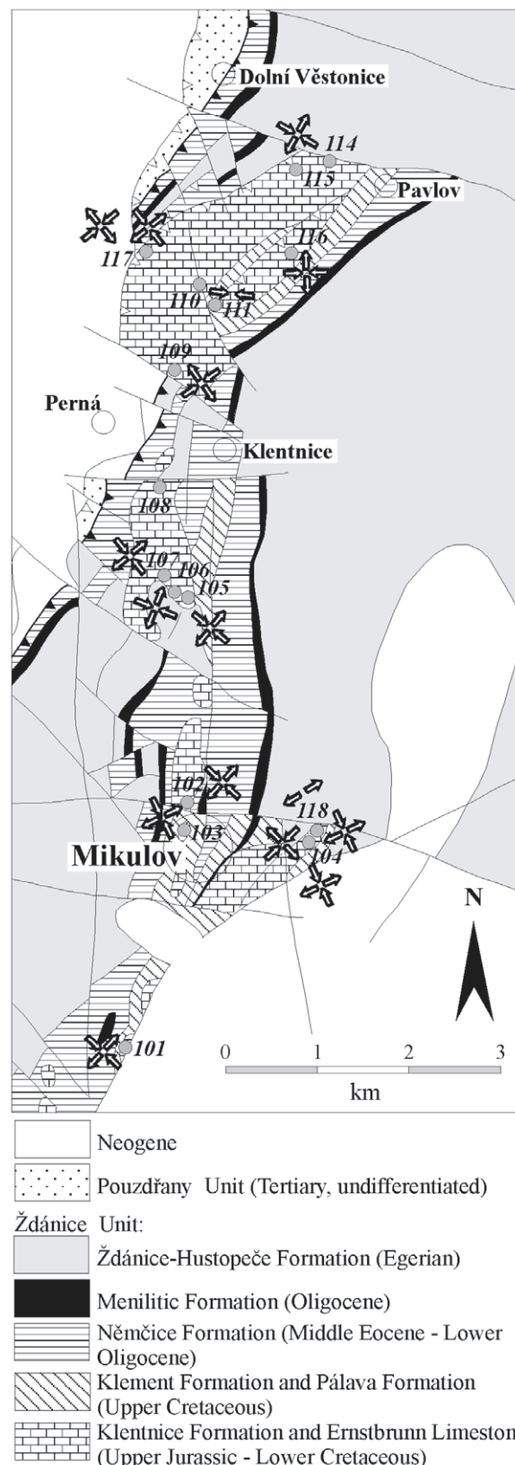
Fig. 3. Geological scheme of the Pavlov Hills region (after Stráník et al. 1999, modified and simplified) with marked studied sites (grey circles). White arrows show computed orientations of horizontal principal stresses (see text for more information).
