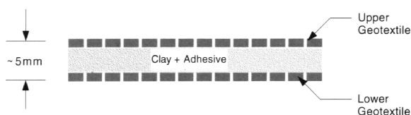
Fig. 1. Cross-section sketch of nonreinforced GCL.
