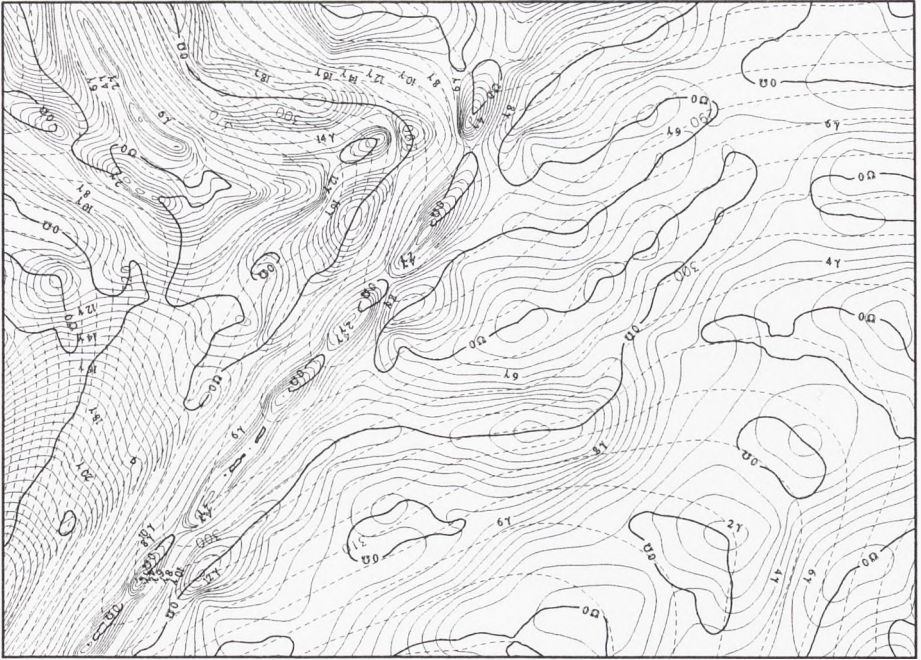
Fig. 1a. \gamma_N and \Omega=0 . Isolines field of slope \gamma_N of georelief in the direction of orthogonal curves to contour lines.
