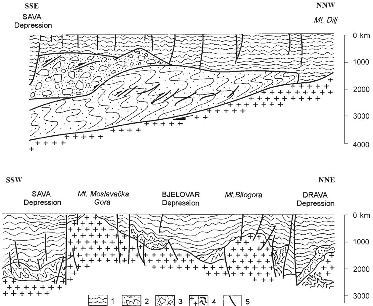
Fig. 5. Geological profiles based on seismical data (Tari-Kovačić & Pamić 1997); profile positions are presented on the geological map — Fig. 1. 1 — Tertiary fill of the Pannonian Basin; 2 — Late Cretaceous–Paleogene sedimentary, igneous and metamorphic rocks of Posavina terrane; 3 — tectonized ophiolite mélangé; 4 — Hercynian crystalline rocks of the Tisia Megaunit; 5 — fault.
