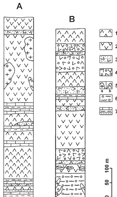
**Fig. 3.** Partial geological columns for the Late Cretaceous volcanic masses: **A** — Mt. Požeška gora; **B** — The Vocin area. 1 — basalt; 2 — rhyolite; 3 — tuff; 4 — volcanic breccia; 5 — small intrusive bodies: a) A-type granite and b) diabase; 6 — Hercynian migmatite; 7 — Upper Cretaceous bedded shale, limestone and sandstone.
