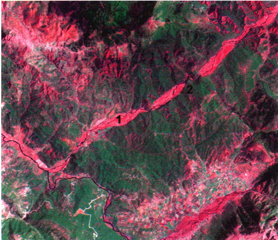
Fig. 5. Sarantaporos River structure with NE-SW direction, material transported by the river and deposited in small basins (1), a small displacement in the river route, due to the activity of a fault, with dextral movement (2).
