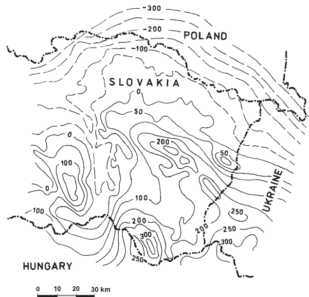
Fig. 2. Bouguer gravity anomaly map of the eastern part of the Western Carpathians (after Ibrmajer 1981 and Šefara 1987). Contour interval 50 \mu\text{ms}^{-2} (5 mGal).
