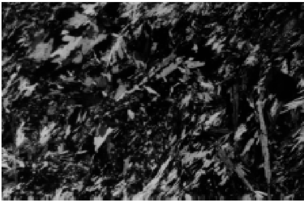
Fig. 2. Random orientation of anthophyllite + hornblende longcolumnar crystals of variable size. Ružindol, magn. 30×, X polars.
