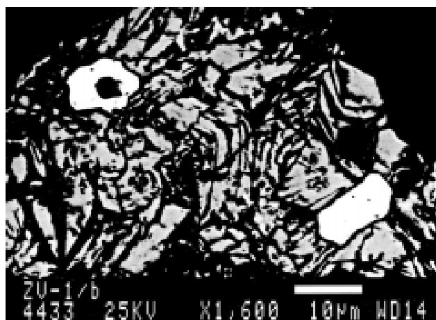
Fig. 9. Section of octahedral crystal of gold (white) in uraninite (grey). ZV 1b, SEM-BEI.
