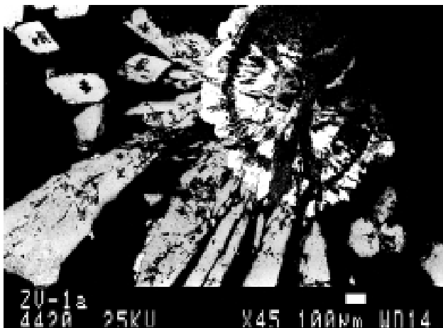
Fig. 5. Radial aggregate of brannerite crystals (grey) overgrowing on zonal uraninite (white) in quartz (black). ZV 1a, SEM-BEI.
