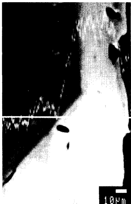
Fig. 12. Back scattered electron image of a grain of a gold-bearing arsenopyrite I crystal with an As-rich rim and line diagram of As content.
