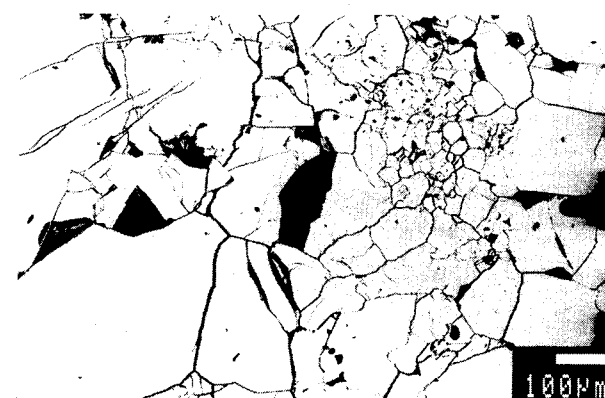
Fig. 15. Brecciated massive structure of arsenopyrite II (light-coloured) in quartz (dark).
