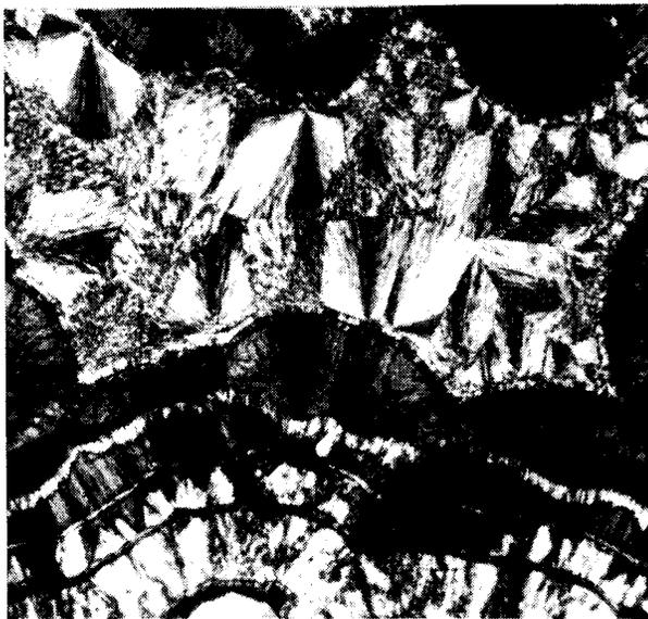
Fig. 6. Typical chalcedony (lenght-fast chalcedony) in the middle part of the infilling of a fissure. Crossed polarizers (XPL), Magn. 35 $\times$ . Loc. Kozárovce.
