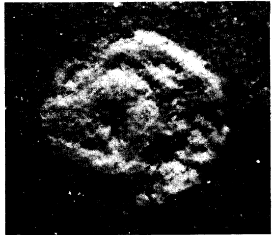
Fig. 11. Calcium carbonate concretion of concentric structure. Sample from 87.8 m. Magnification 35 \times .
