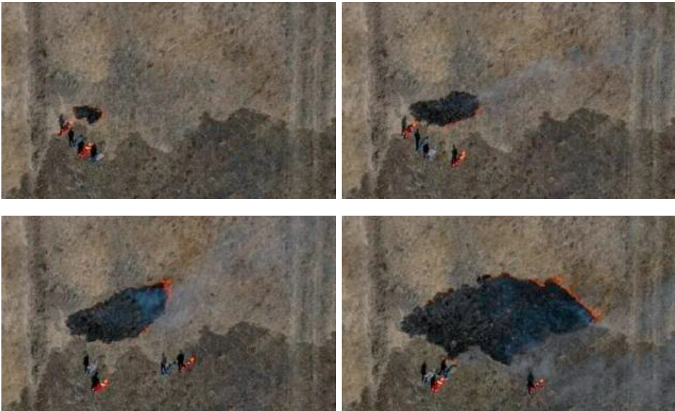
FIGURE 4. Image data from quadcopter. Propagation of the first fire perimeter used in the following experiments.
