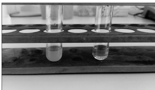
Figure 1. Examples of methanol extract of human hair following centrifugation. The second, clear sample was performed using present methodology.
