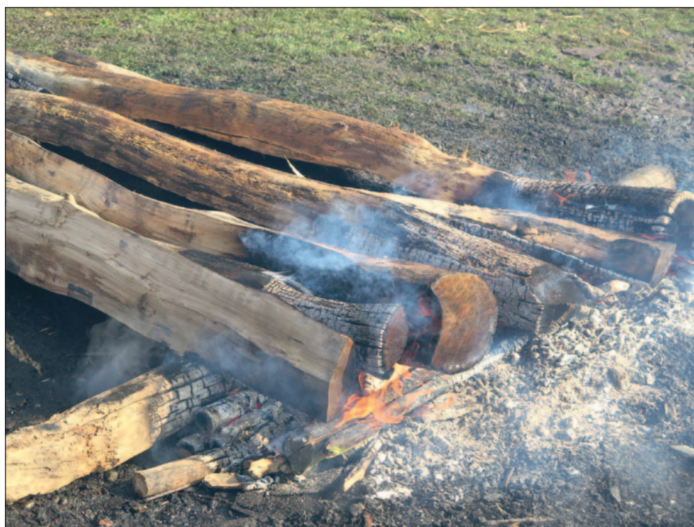
Fig. 6. Modrá. Charring lower parts of oak beams.
