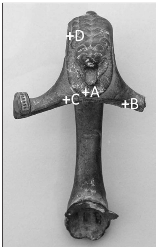
Fig. 4. Localization of non-invasive Raman measurements of white incrustation (A), green patina (B) and localization of extraction of sample for SEM-EDS analysis of pure alloy (recent surface damage – C) and black patina (D).
