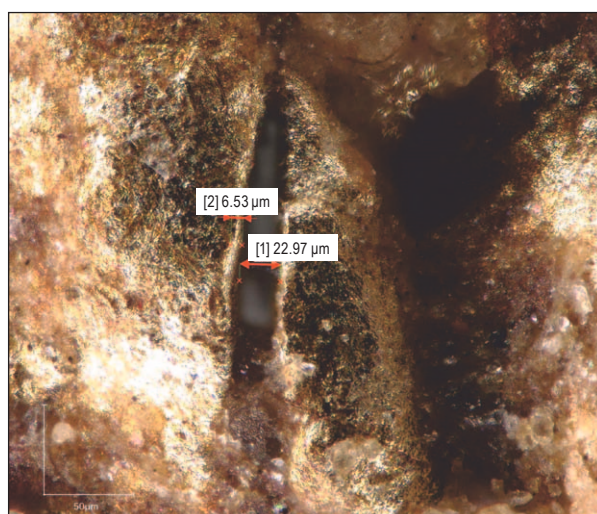
Fig. 14. Fragment No. 1. Digital measurement of the wire of twisted sheet metal strip – width of the seamline and thickness of sheet metal strip.
