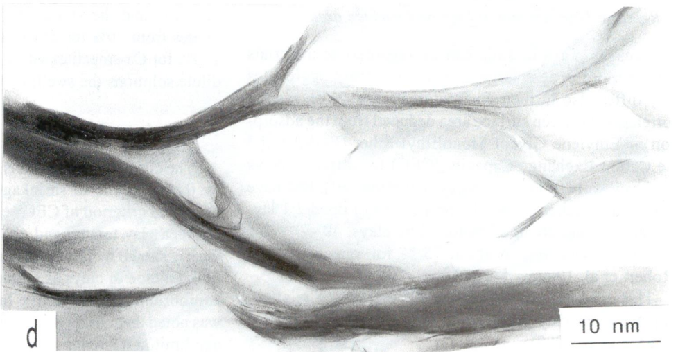
Fig. 3. Bulk volume and microstructure of Greek montmorillonite prepared with 1M NaCl solution at 0.0032 MPa (a), 0.1 MPa (b), and 1MPa (c), where w = water content and e = void ratio ( V_v/V_s ). Channels between pores at 0.1 MPa are illustrated in (d) (from Tessier 1984).
