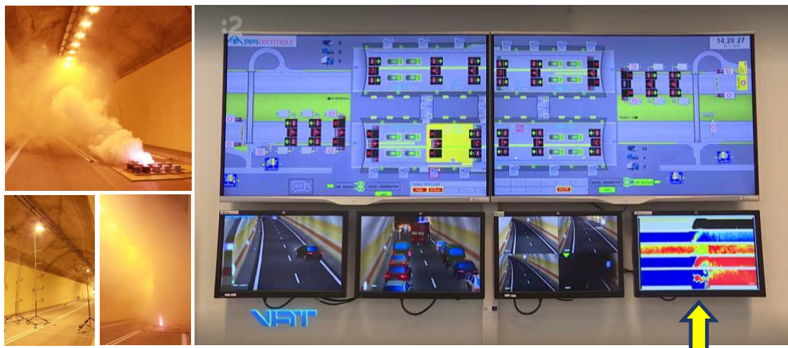
Full-scale smoke tests in real motorway tunnels (left) and visualizations integrated in the screen 6 in TTOS (photo from Science&Technology telecast about TTOS in RTVS) (right).
