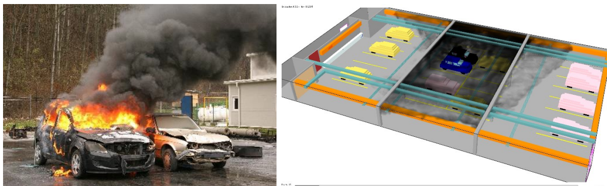
Computer simulation of automobile fire and automobile fire in car park.
