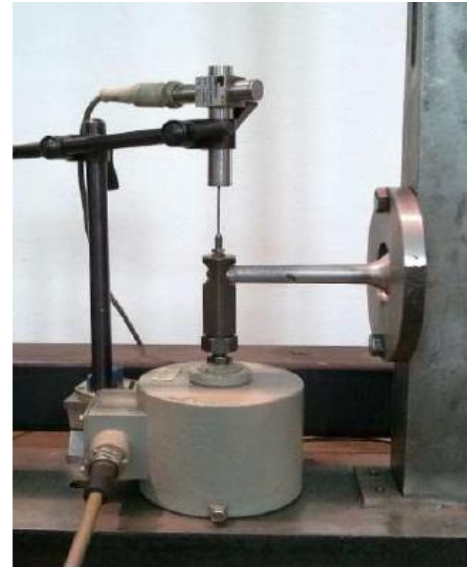
Cantilever made of composite (left) and Mg alloy, bending test on cantilever (right).
