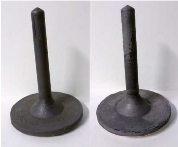
Cantilever made of composite (left) and Mg alloy, bending test on cantilever (right).
